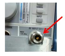
(Spectrum analyzer with N-type to connect RF cable)
